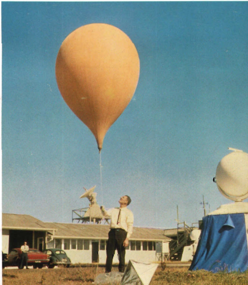
Launching a radio-sonde balloon from the Laverton weather station. Bureau of Meteorology
